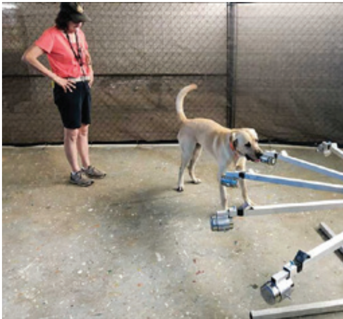
The training aid delivery devices (TADD) attached to each arm of the wheel allow the dog to safely detect the substance inside without being exposed to the substance. Photos courtesy United States Army
