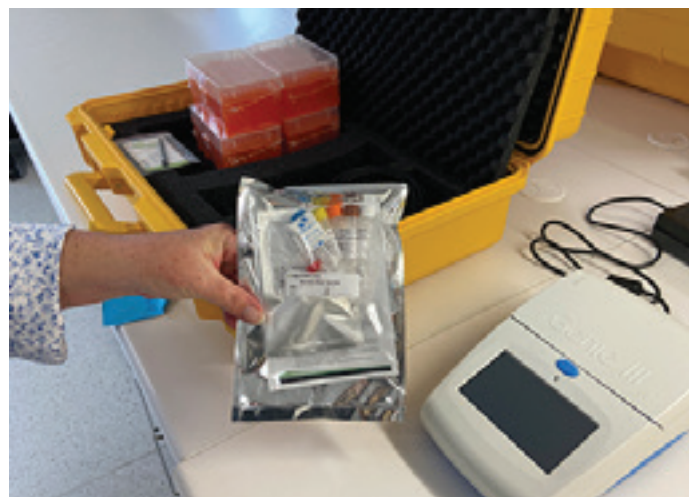
A ready-to-go Hendra virus test kit, along with a LAMP Genie III diagnostic machine, which together can diagnose Hendra virus in horses in under an hour.
